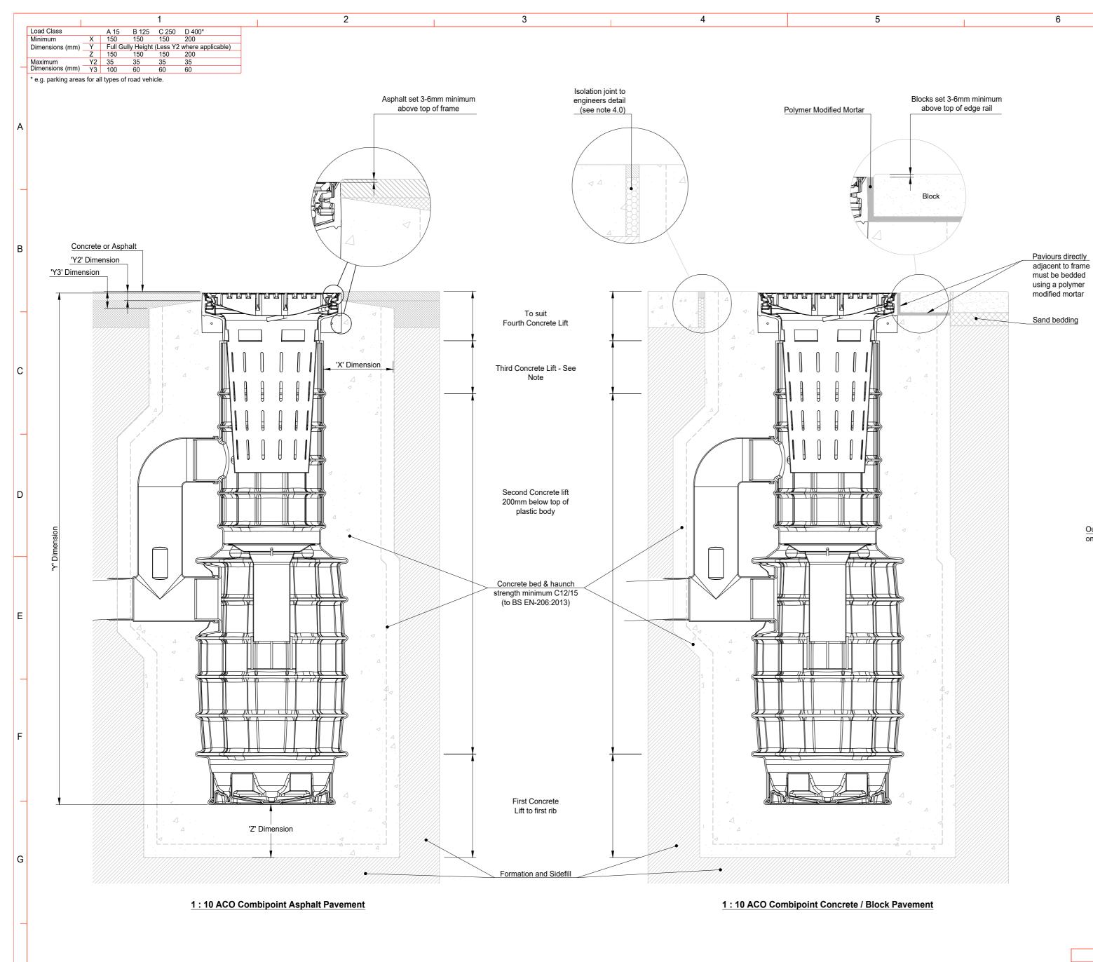
1.0 Load Class Installation recommendations shown are ACO minimum recommendations for BS EN 1433:2002 load class requirements.
