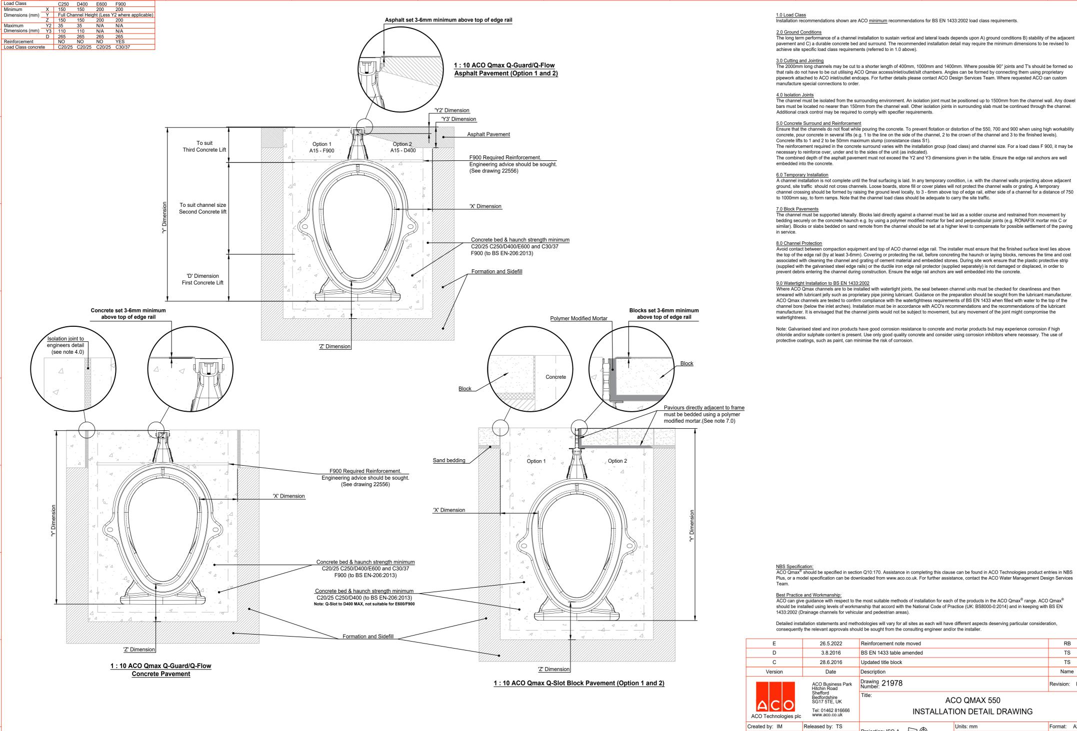
The long term performance of a channel installation to sustain vertical and lateral loads depends upon A) ground conditions B) stability of the adjacent pavement and C) a durable concrete bed and surround. The recommended installation detail may require the minimum dimensions to be revised to
