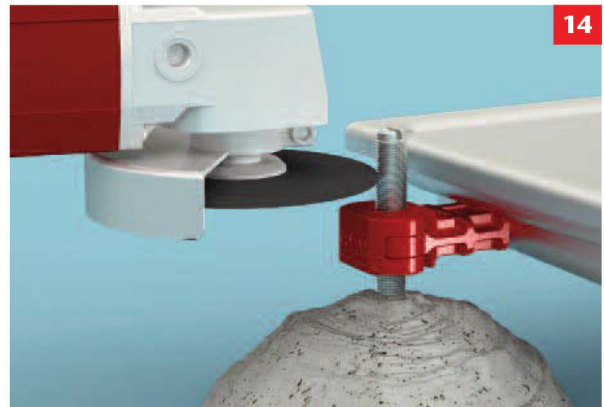
If the threaded post of the levelling feet interferes with the intended floor level cut the post down to appropriate level. Please cover the channel to prevent steel particles cross contaminating the stainless steel, as this can cause corrosion in the future.
