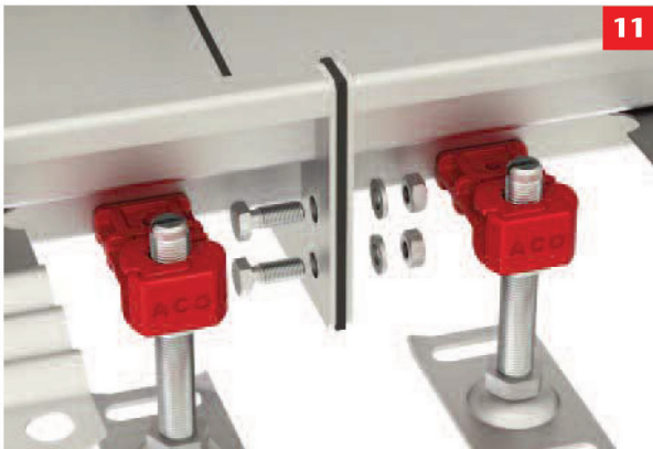
Align gasket and end plates of the channels and insert the bolts through the holes. Hand tighten the nuts on the bolts.
