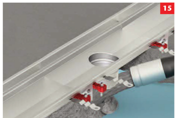
For light and medium duty applications (up to load class C250) a suitable mortar of Strength Class 30/37 to BS EN 206-1 with a minimum aggregate size of 10mm should be used.
