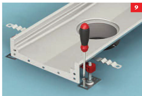
Once channel is in place fasten the levelling feet to the ground.
