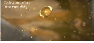
The Coalescence gap accelerates the FOG droplets causing them to collide and coalesce into bigger droplets that separate out of the waste water more efficiently.
