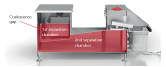
Patented two separation chambers. The first chamber for separation of FOG restricts flow and forces the FOG toward the coalescence gap.
