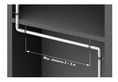
As a guide, use the table below for bracket spacing on horizontal pipes.
