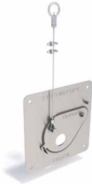
ACO Q-Plate with remote draindown and bypass recommended for all orifice apertures less than 100mm
