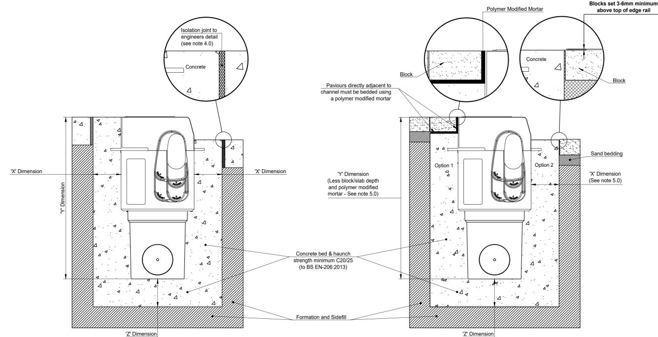
1: 10 ACO KerbDrain Gully Concrete Pavement
